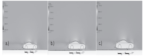
Fig.8 Velocity distribution contours adding rear spoiler at: a) 100km/hr., b) 180km/hr. and c) 240km/hr.
