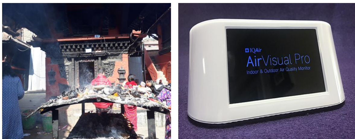
Figure 2 (a) installation of device in the temple (b) the instrument used: Air Visual Pro
