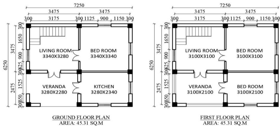
**Figure 8:** Ground floor and first floor plan BMC 2.3 RCC
