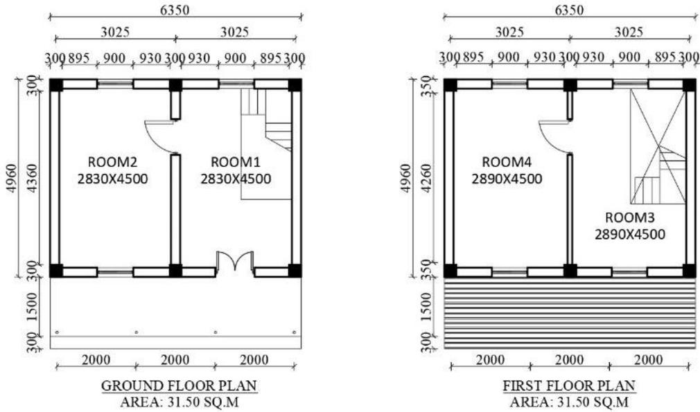
**Figure 4:** Ground floor and first floor plan BMC 2.1 RCC
