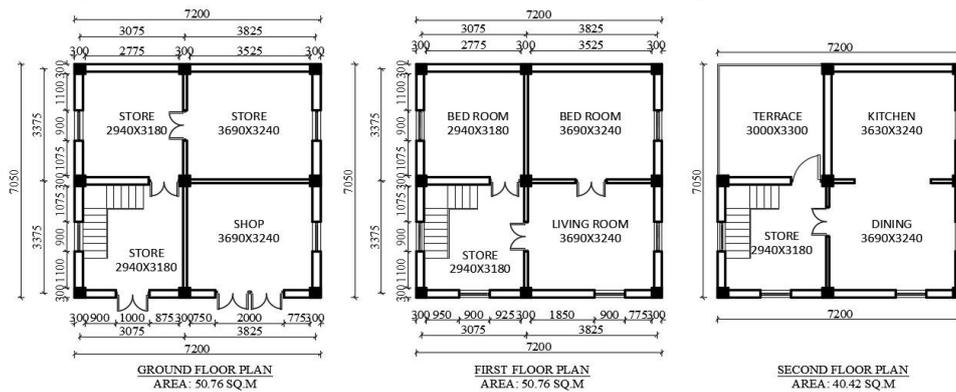
**Figure 10:** Ground floor, first floor & second floor plan BMC 2.4 RCC
