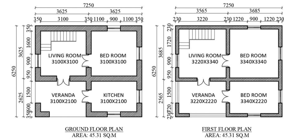
**Figure 7:** Ground floor and first floor plan BMC 2.3 LB
