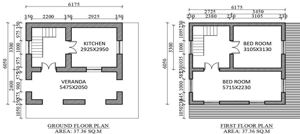
**Figure 5:** Ground floor and first floor plan BMC 2.2 LB
