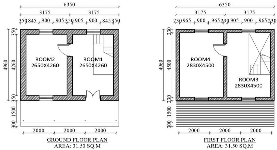
**Figure 3:** Ground floor and first floor plan BMC 2.1 LB
