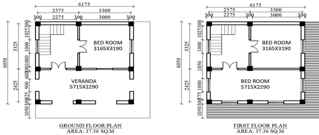
**Figure 6:** Ground floor and first floor plan BMC 2.2 RCC
