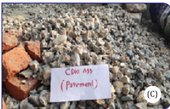
Figure 3: Recycled Aggregate: (a) Recycled Concrete Aggregate from Waste Concrete Cube Specimen (b) Recycled Concrete Aggregate from Demolished Building (c) recycled Concrete Aggregate from Demolished Road Pavement (d) Recycled Brick Aggregate from Demolished Building
