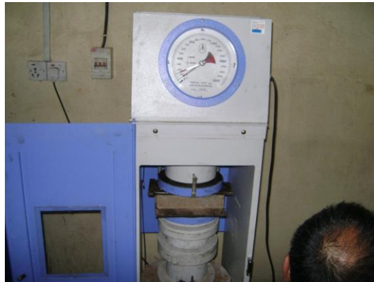
Figure 1: Test of dry compressive strength of CSEB unit ((Bhatt, 2015))
