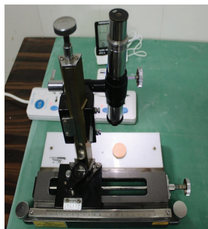
Figure 4: Measurement of test specimen by travelling microscope
