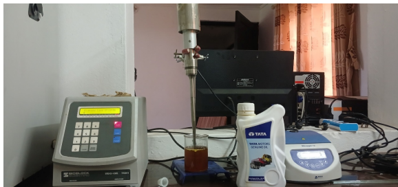
Figure 3: Ultra-sonication for preparing hybrid Nanofluid
