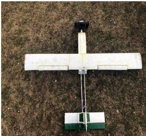
Figure 8: Final assembled glider
