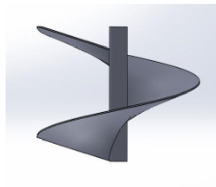
Figure 5: Proposed Screw turbine model
