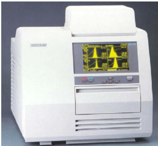
Fig 1: TLD Harshaw 6600 plus model
