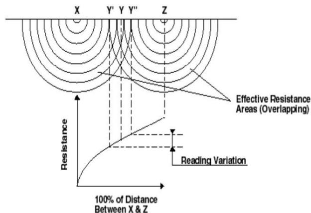
Figure 4: Schematic diagram for working of auxiliary rod. [Adapted from 15, 16]
