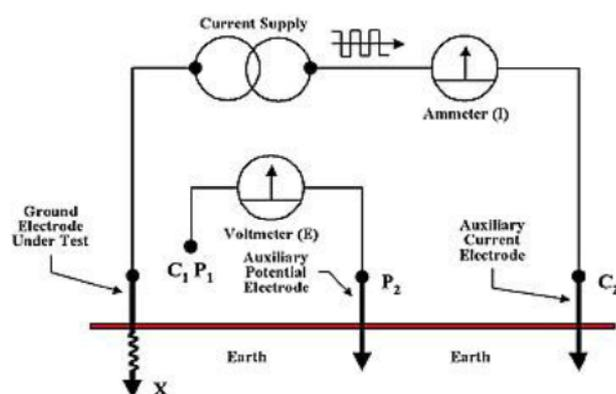
Figure 3: Schematic diagram for the measurement of the ground potential. Adapted from [15].
