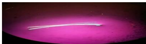
Figure 3: Microscopic viewed image of asbestos fiber when parallel polarized light passed before treatment.
