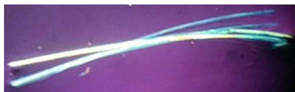
Figure 4: Microscopic view image of asbestos fiber when perpendicular polarized light passed before treatment.
