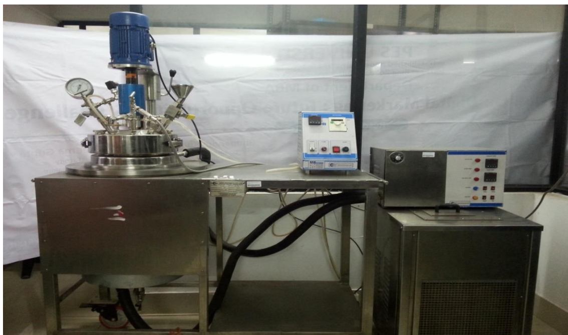
Fig 3: Pilot plant for production of biodiesel from Waste Vegetable Oil
