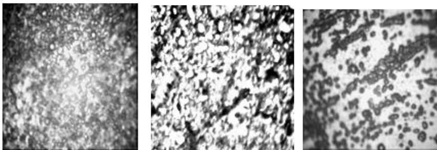
Figure 3 (a-c): Micrographs of HAZ Samples at Slow, Moderate and Fast Speeds Respectively after Etching in Solution of 1 ml HCl + 3 ml HNO 3 + 1ml Glycerol at 400 xx.
