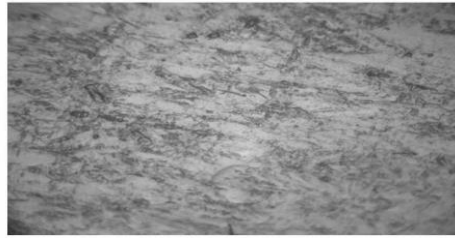
Figure 2: Micrograph of As – received Sample after Etching in Solution of 1 ml HCl + 3 ml HNO 3 + 1ml Glycerol at 400 xx.
