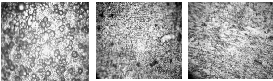
Figure 2: Micrograph of As – received Sample after Etching in Solution of 1 ml HCl + 3 ml HNO 3 + 1ml Glycerol at 400 xx.
