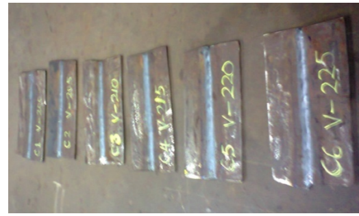
Figure 1: Finished welded test plates with 200 × 100 × 5 mm dimensions.
