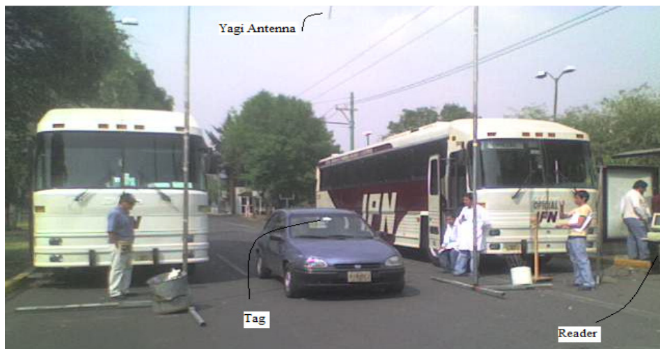
Fig. 7 The buses form a dielectric wall.
