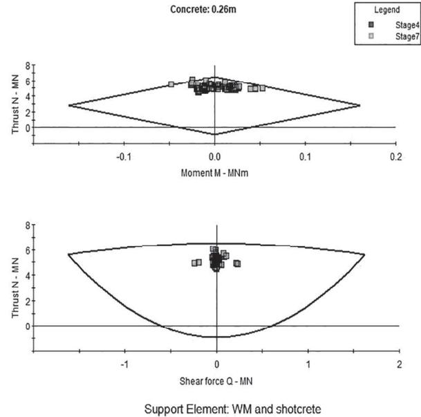
**Figure 23: Support capacity plots for shotcrete (stage: Full face excavation and application of revised support)**
