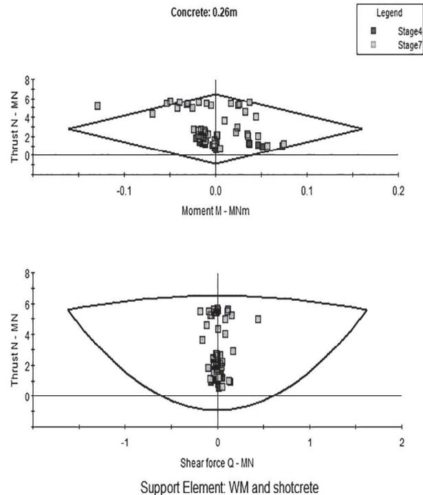
Figure 20: Support capacity plots for shotcrete (stage: excavation and application of revised support in the top heading part)
