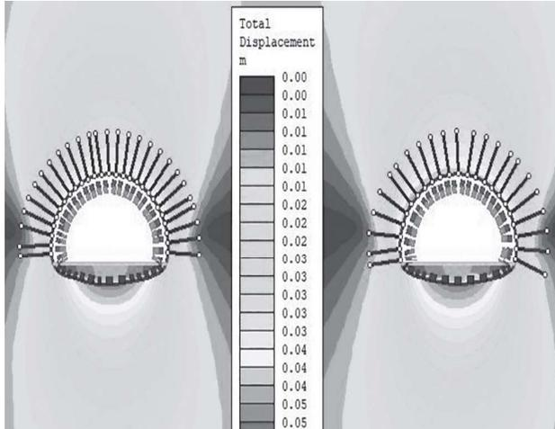
**Figure 21: Total displacement contour after installation of support (stage: full face excavation and application of original support)**
