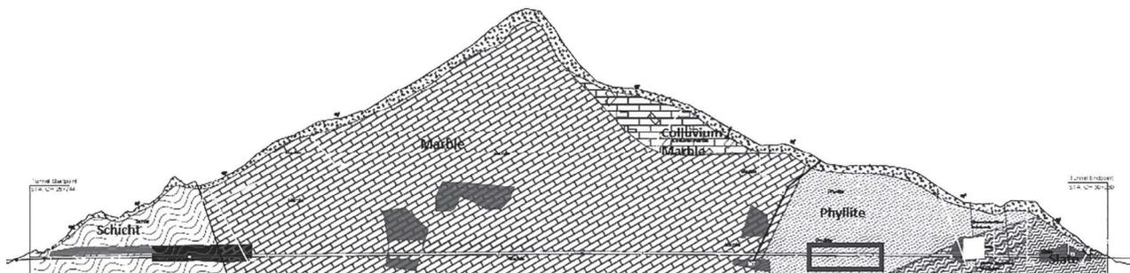
Figure 2: Geological profile along Mahadevtar tunnel, problematic area marked in red, pink patches represent water rich strata (Source: China State, 2021)
