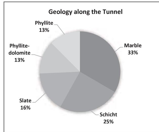
Figure 1: Geology along the Mahadevtar Tunnel
