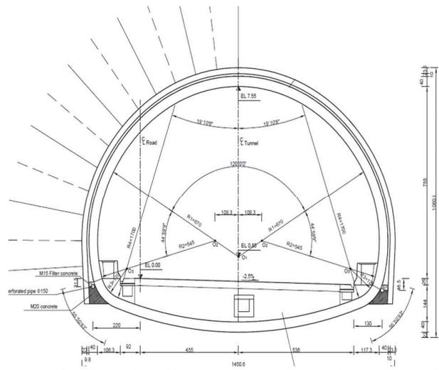
**Figure 5: Tunnel cross section with support measures for support class P4-2 (Source: China State, 2021)**
