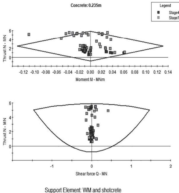
Figure 19: Support capacity plots for shotcrete (stage: excavation and application of original support in the top heading part)
