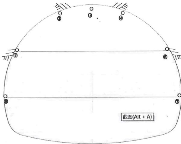
Figure 15: Monitoring points in Ch. 29+299
