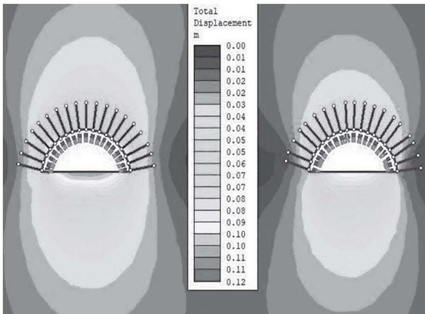
Figure 18: Total displacement contour after installation of support (stage: excavation and application of original support in the top heading part)
