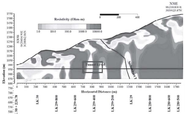
**Figure 3: MT survey result- Resistivity diagram -the problematic area is marked in blue (Source: China State, 2022)**
