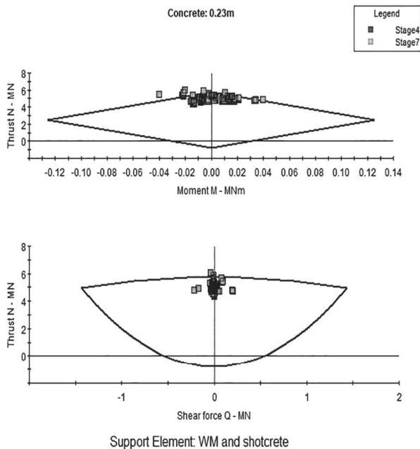
**Figure 22: Support capacity plots for shotcrete (stage: Full face excavation and application of original support)**
