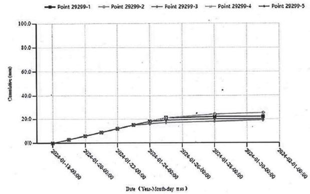
Figure 16: Monitoring data of the Tunnel at Ch. 29+299
