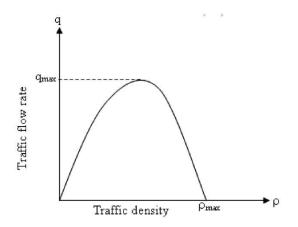
In this diagram, the slope is positive until the maximum flow rate,  $q_{max}$ , is reached, and negative thereafter.
