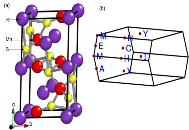
**Fig. 1:** (a) Crystal structure of  $K_2Mn_3S_4$ ; (b) 3-D Brillouin zone of  $K_2Mn_3S_4$ . The red dot indicates the high symmetry point in the momentum space.
