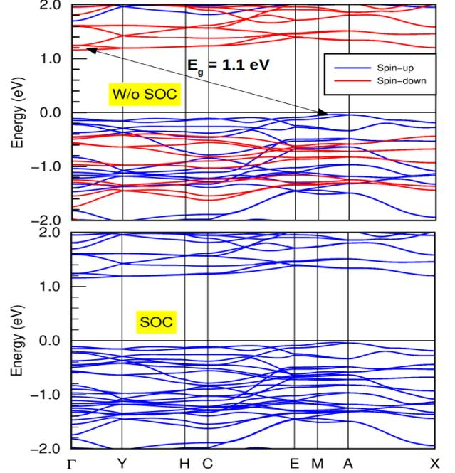
**Fig. 3:** Electronic band structure of  $K_2Mn_3S_4$  in scalar (top) and full-relativistic (bottom). Horizontal solid line indicates the Fermi level. Arrow denotes the indirect band gap between the high symmetry point that lies in the different energy of the momentum space.
