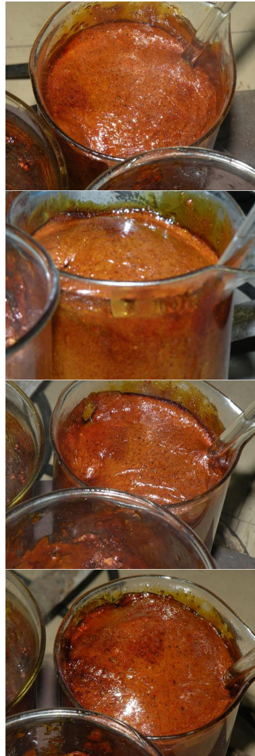
FIGURE 2. Puffy and porous ZNCF samples obtained after co-precipitation.
