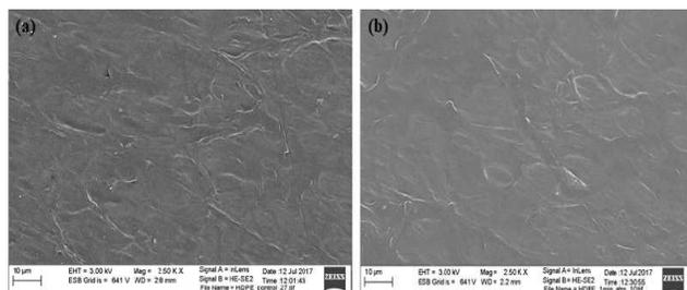
**FIGURE 5.** SEM image of (a) control and (b) plasma jet treated samples of HDPE
