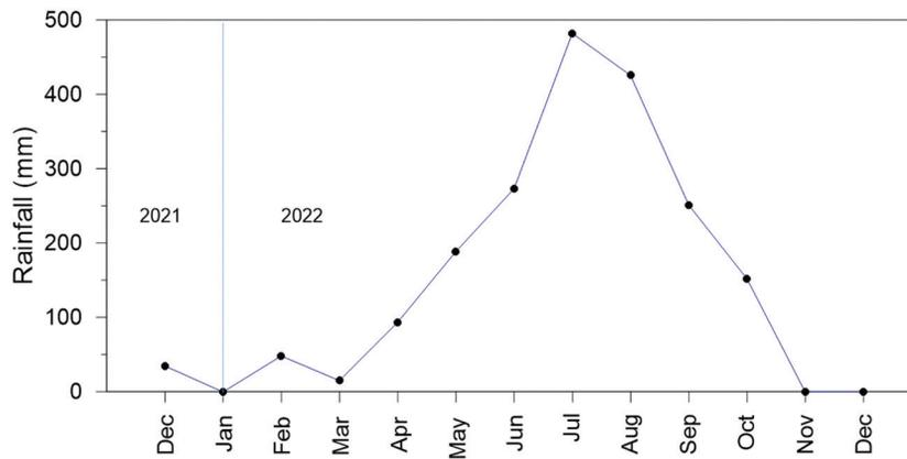
**Fig. 10: Monthly rainfall data (DHM, Nepal), recorded at the nearby Thokarpa gauge station, to the Dutti landslide.**
