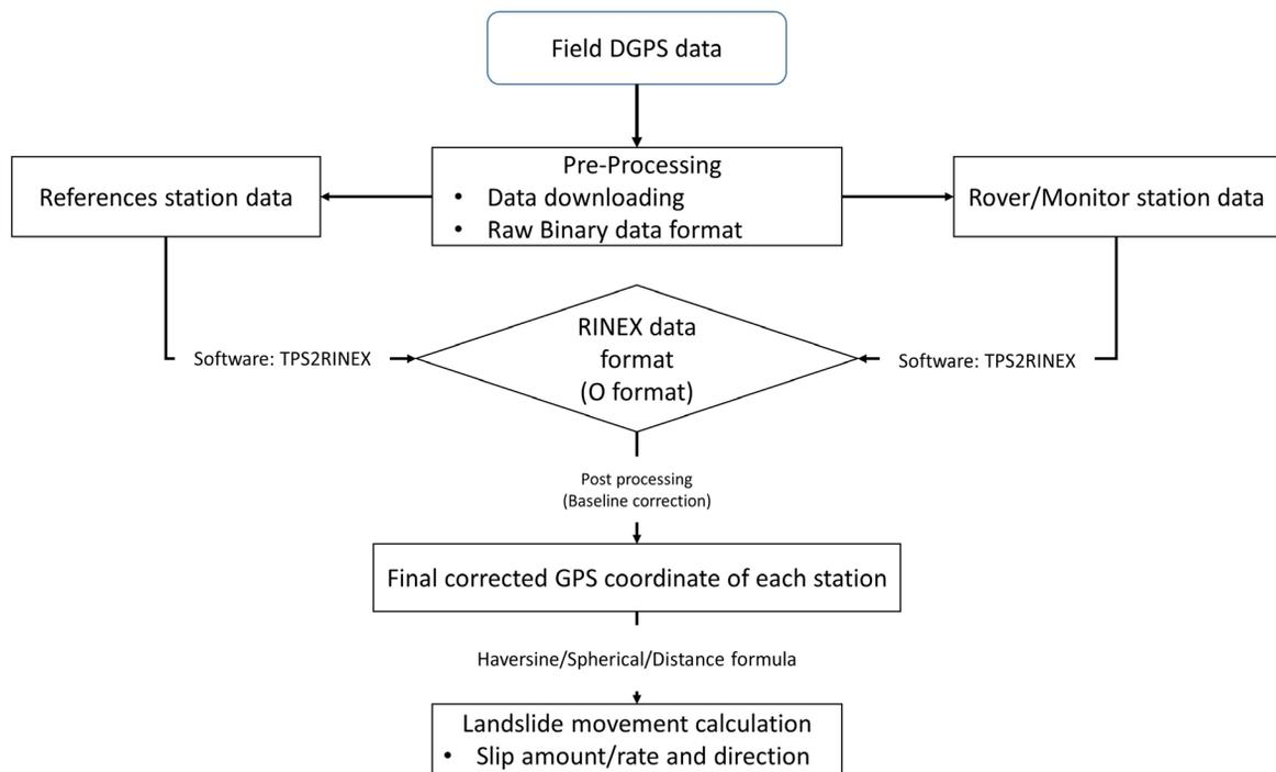
Fig. 6: Flow diagram of the processes used for the analysis of GPS data.
