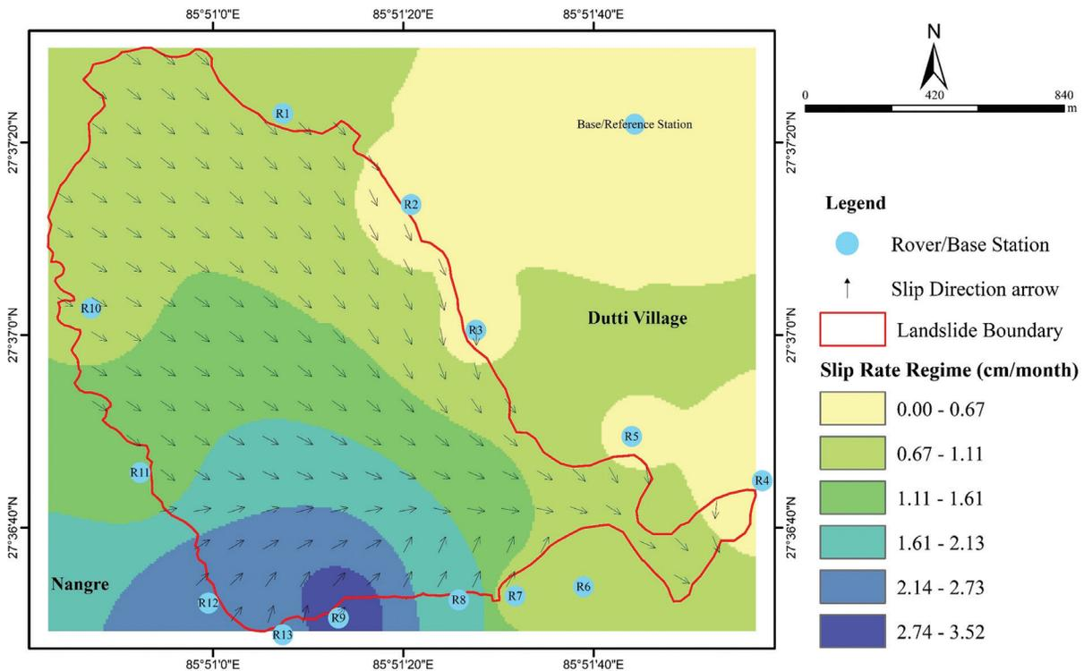
Fig. 9: Map shows slip rate and slip direction of the Dutti Landslide.
