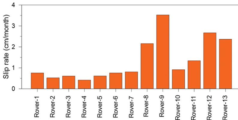
Fig. 8: Average monthly slip rate at each rover station established in the Dutti landslide.
