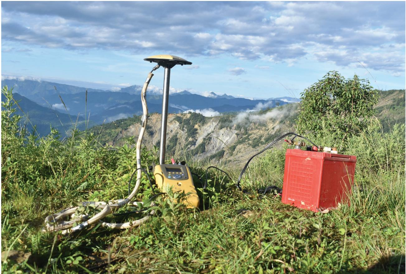
Fig. 5: Data acquisition by Topcon GPS receiver in the field.
