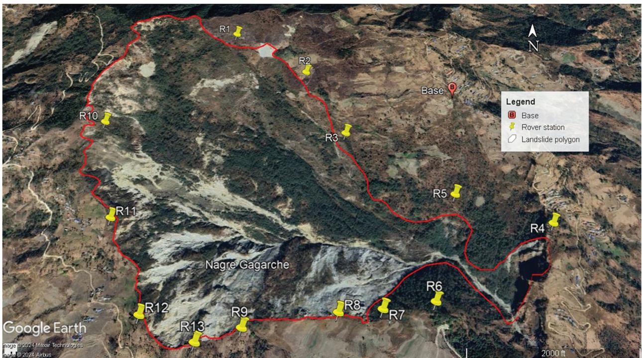
Fig. 3: Location of rover GPS and base stations at the Dutti Landslide.
