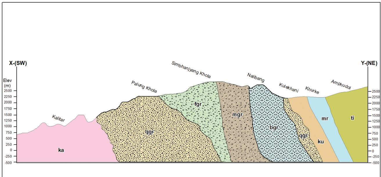
Fig. 4: Geological cross section along X and Y. Four zones of the granitic body are shown through this section.
