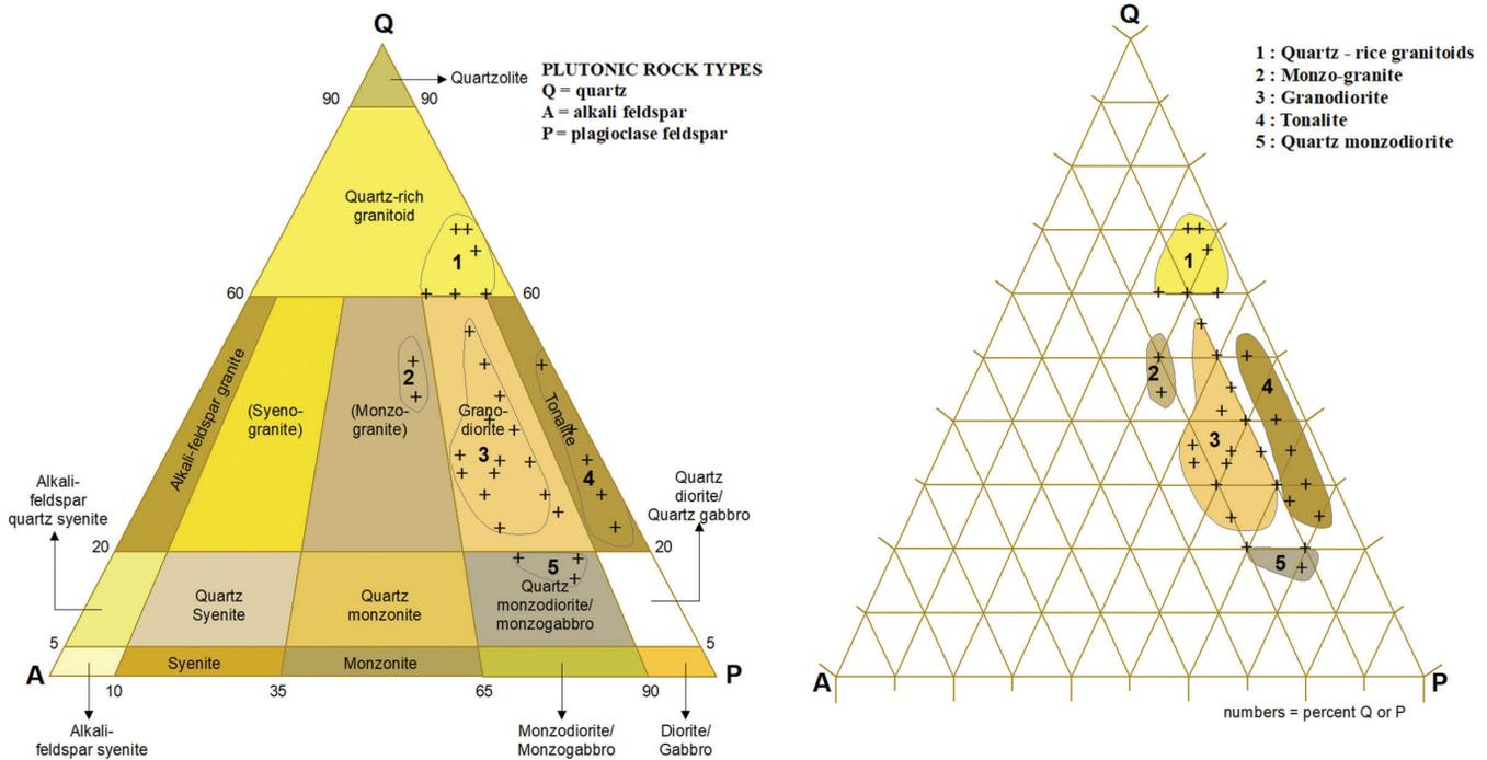
**Fig. 8:** QAP diagram showing the sub-classes of the Palung Granite based on an essential mineral percentage (the left figure is the standard classification proposed by Streckeisen, 1973, and the right one is the present work). See supplementary tables used for the classification in Annex 1, Tables 1-3.
