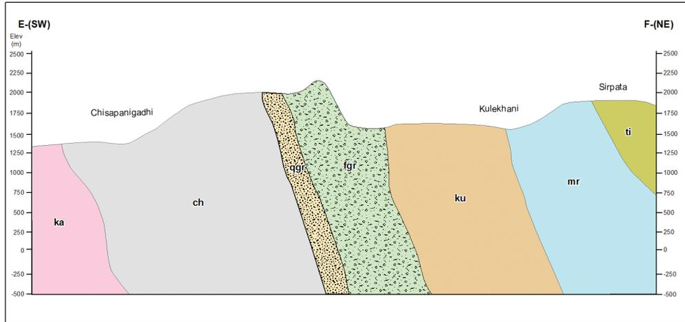
Fig. 5: Geological cross-section along E and F. Two zones of the granite body are distinct in this section.
