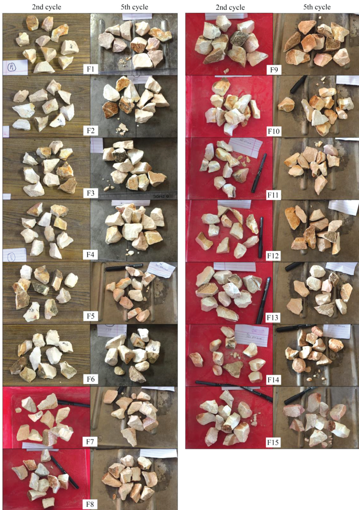
Fig. 8: Deterioration at 2 nd and 5 th cycles of slake durability test of quartzites from the Fagfog Quartzite. Samples F1, F2, F3, F4, F5, F10, F12 and F13 undergo type I deterioration and the remaining samples undergo type II deterioration.
