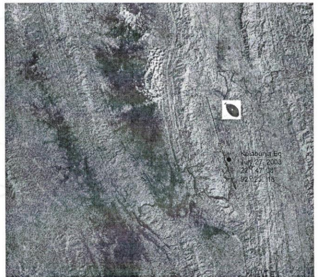
Fig. 7: The Kolabunia (Rangamati) earthquake of 2003 July 27 with its epicentre location ( 22^{\circ} 47' 08'' N, 92^{\circ} 23' 18'' E), moment tensor magnitude 5.6, and focal depth of 11 km. The event occurred along the clay-rich fault zone. The fault plane solution suggests a major thrust with a minor strike slip.
