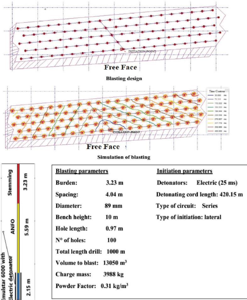
Fig. 3: Blasting data and Simulation of blasting.
