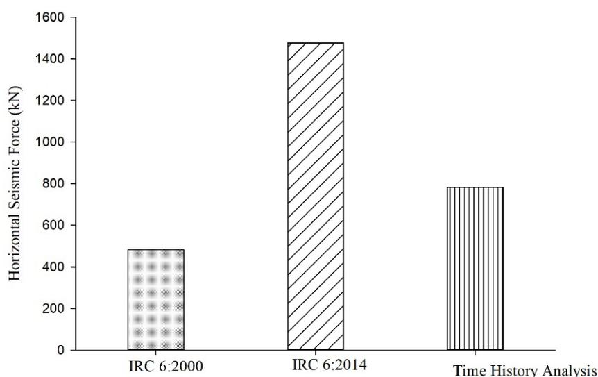
**Fig. 5: Comparison of horizontal seismic load obtained from codes and time history analysis**
