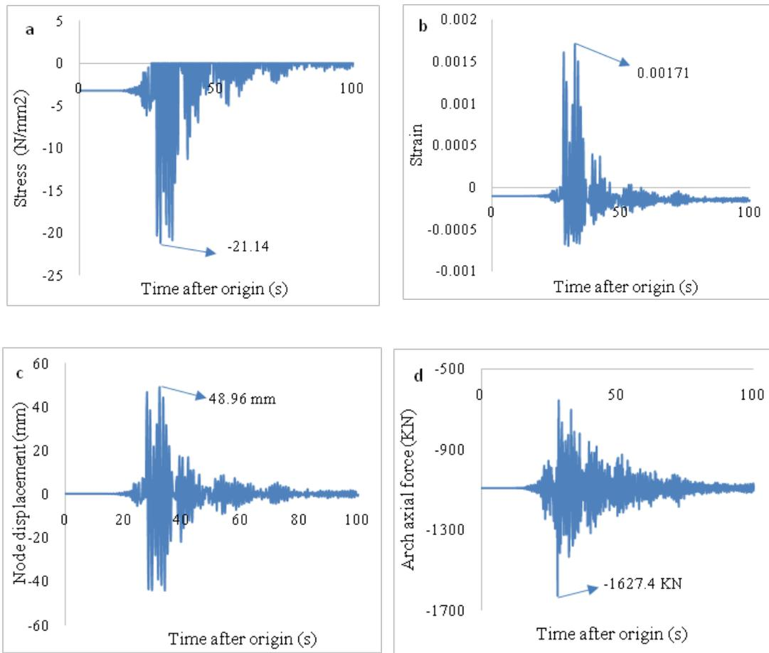
**Fig. 4: Response quantities during Gorkha earthquake; a) Stress variation b) Strain c) Node displacement d) axial force fluctuation in arch rib.**
