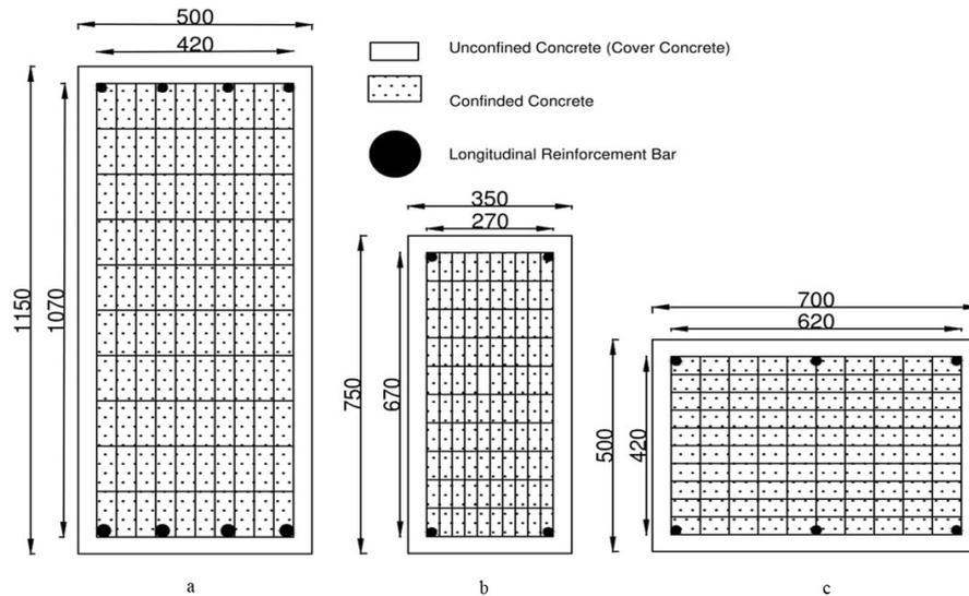
Fig. 2: Fiber section used; a) Arch b) Arch cross beam c) Column
