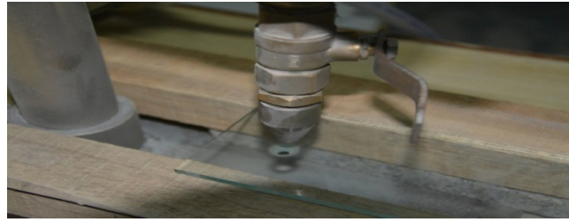
Fig.1: Hole generated by Abrasive jet machining process
