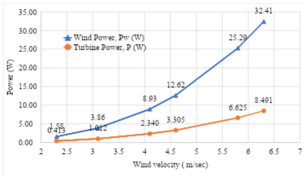
Figure 5: Wind Power vs Turbine Power
