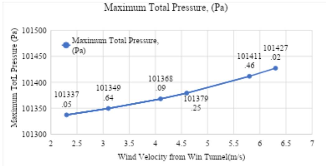
Figure 7: Maximum Total Pressure vs Wind Tunnel Velocity
