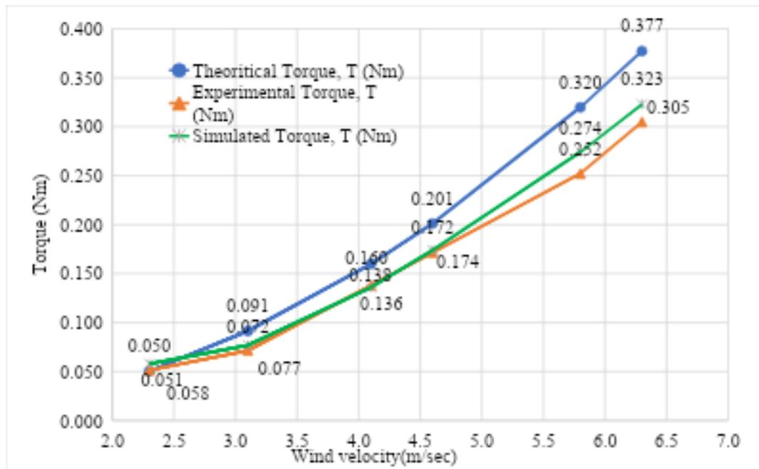
Figure 10: Theoretical Torque vs Simulated Torque vs Experimental Torque
