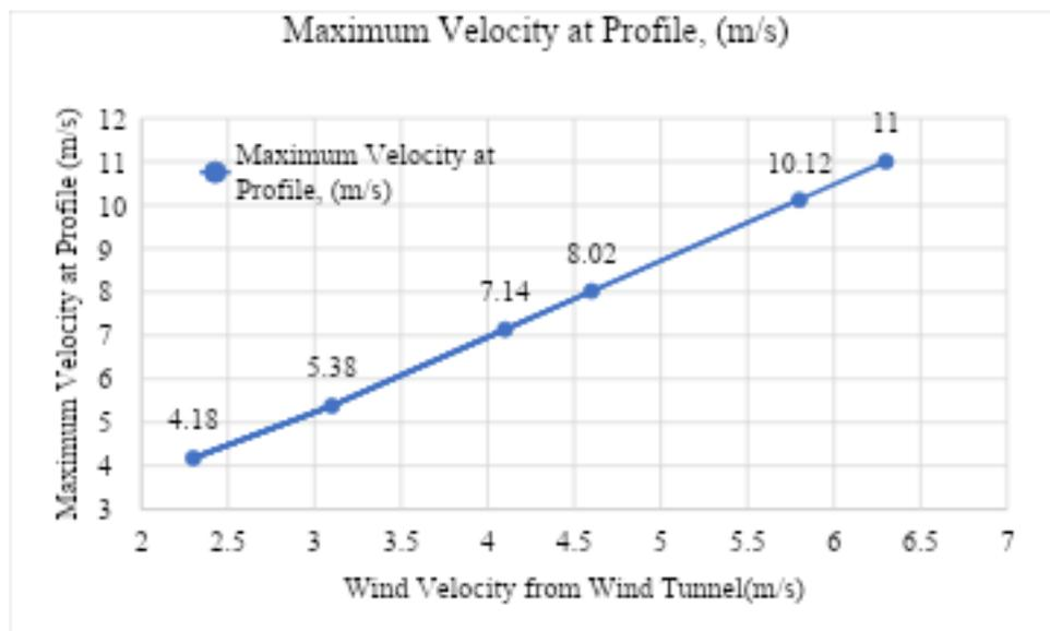
Figure 6: Maximum Velocity at Profile vs Wind Tunnel Velocity
