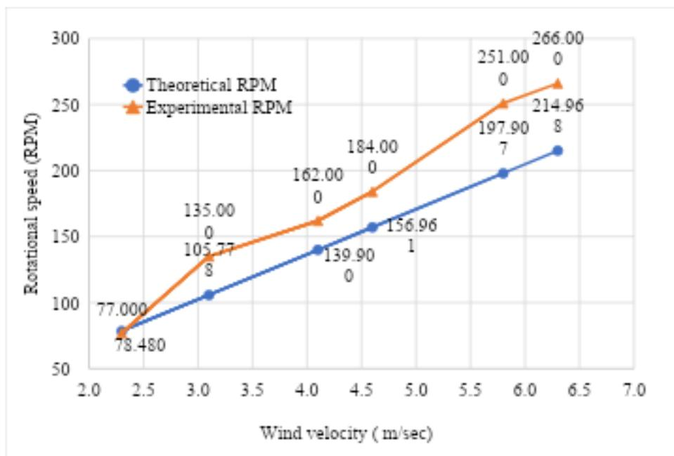
Figure 9: Theoretical Rotational Speed vs Experimental Rotational Speed
