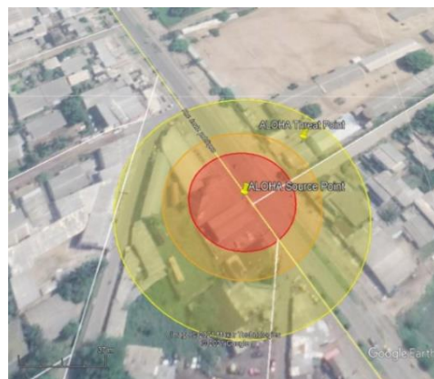
Figure 10b Thermal radiation threat zone from pool fire in the rainy season
