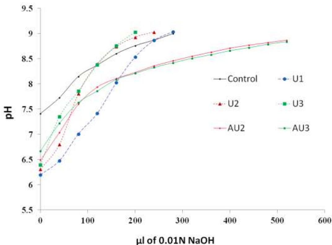
Fig. 2: Effect of urea and Biochar on the buffering capacity of soil samples collected on day 1
