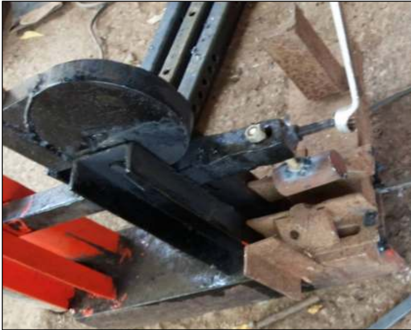
Fig. 7 Developed jig for bending float.
