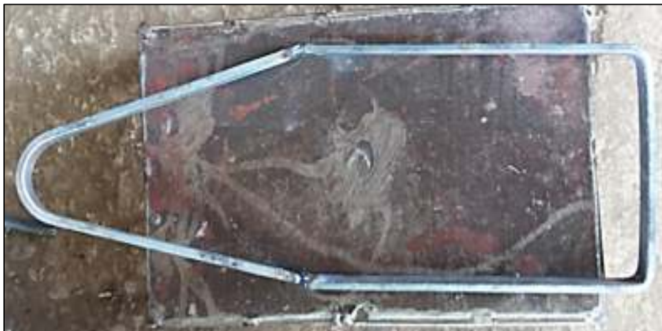
Fig. 10 Frame manufactured by jigs & fixtures
