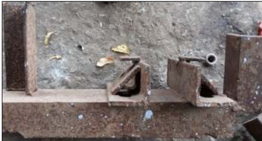
Fig. 6 Developed fixture for bending the float
