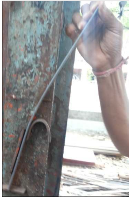
Fig. 2 Hand-made jig for bending float
