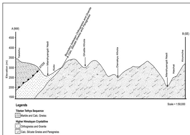
Fig. 3: Geological cross-section from A (Talekhu) to B (Krumche)
