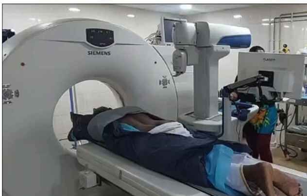
Figure 4: Patient being docked on computed tomography table with MAXIO robotic system
